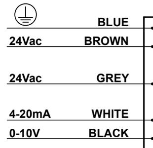
To control the opening and closing of the zone valve through the actuator, simply connect the blue cable to neutral, the brown cable to phase and the black cable to the 0-10V control unit (or the white cable if the regulation is 4-20mA). The grey cable is used to invert the starting point of the actuator and, as far as our applications are concerned, we suggest to leave it always under power.
